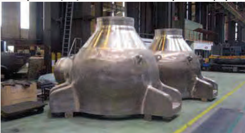
Primary pump casings ( www.aveva.com )
