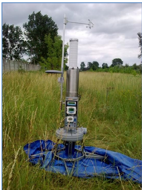
Fig. 6. The mobile aerosol sampling and measuring station at work
