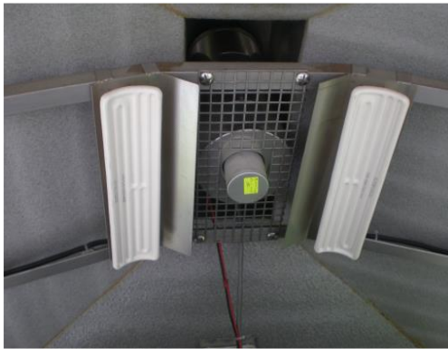
Fig. 3. NaI(Tl) detector and heating of the filter [1]
