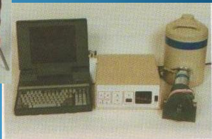
Figure 4 MCRS: Medium Count Rate Plutonium Isotope with Ge detector.
